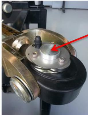
Bi-lock pin installed in DO35 coupling (Top View)
